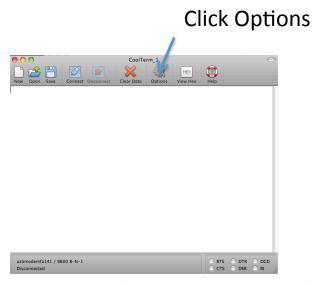
Make sure the Baudrate is set to 9600 (remember, in Arduino we set it to 9600 using Serial.begin(9600)
