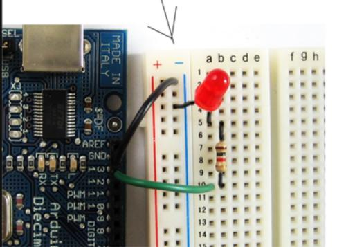
NOTE: RESISTORS can be connected EITHER way (unlike LED's)
